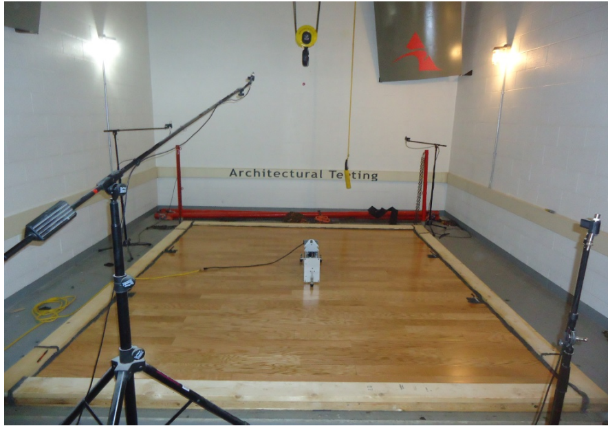
Source Room View of Test Specimen Installation
