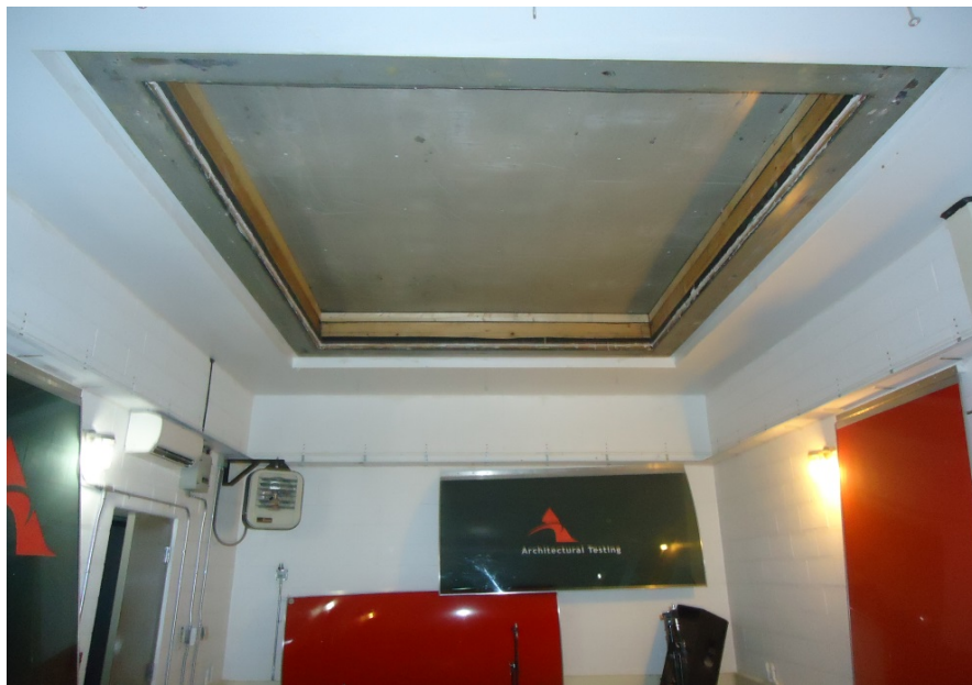
Receive Room View of Test Specimen Installation
