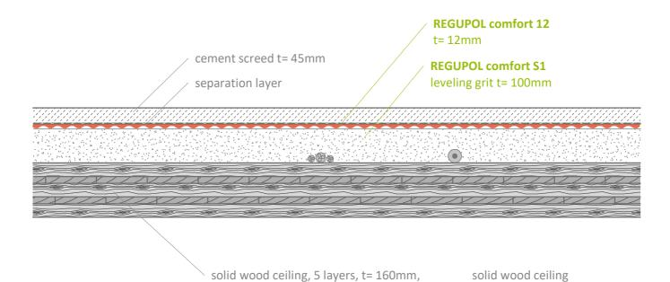
made of laminated wood ED-BSP, longitudinal layers t= 40mm, transverse layers t= 20mm
