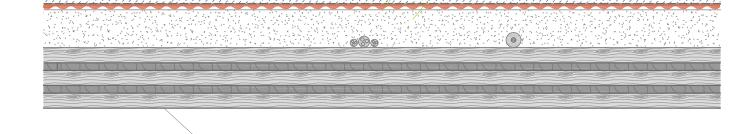
solid wood ceiling, 5 layers, t= 160mm, made of laminated wood ED-BSP, longitudinal layers t= 40mm, transverse layers t= 20mm
