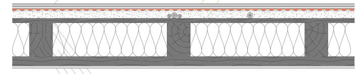
ceiling formwork wooden beam insulation battening drywall
